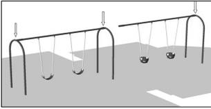
**PROBLEM:** The welded connection of the sleeve joint to the arch support can crack or break. When this happens, the top swing beam can collapse causing children on the swings to fall and be injured.
